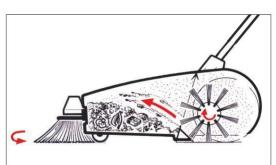
The side broom sweeps dust and debris from corners, directly into the path of the wide main broom, which in turn flips the same into the large self collecting hopper.
