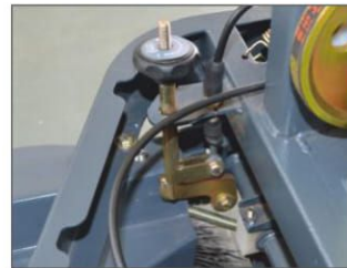
Easy access to broom adjustment system
