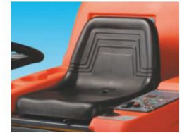
Ergonomically designed driver seat for comfort, easy access to all controls and good all round visibility.
