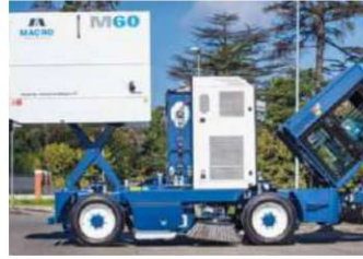
Dumping at any height between 1,1 and 2,3 m.
