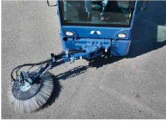
Fully adjustable third front brush that allows to sweep 180° left and right side.
