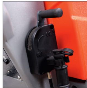
Parking brake to hold the machine during operation for safety.
